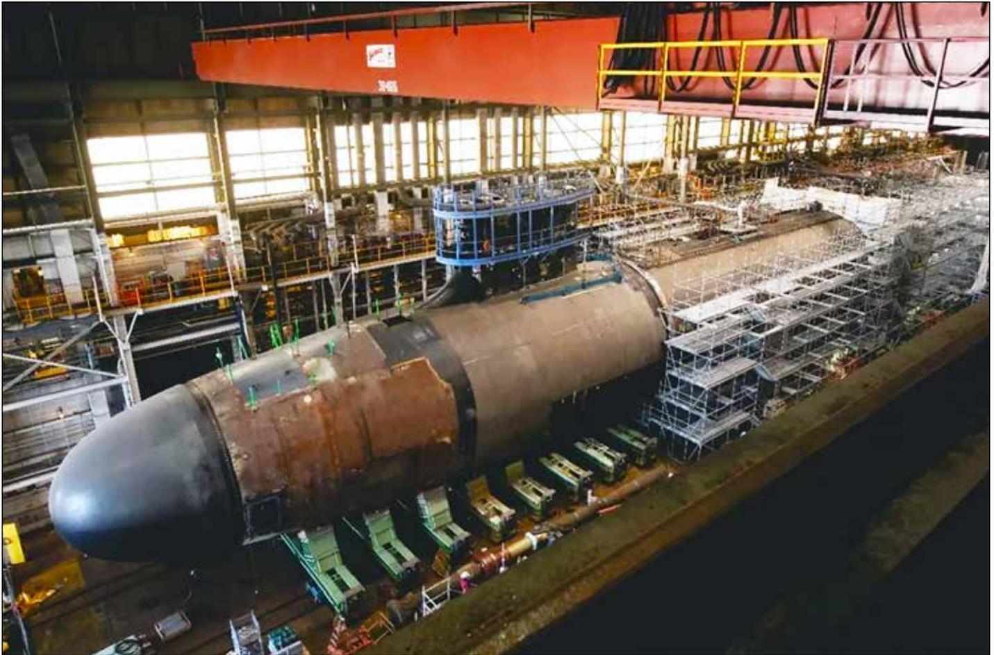
*Virginia-class submarine, USS Arkansas (SSN-800) is now pressure hull complete, which means all parts of the hull are joined and watertight. (Photo Credit: Ashley Cowan/ HII.)*
