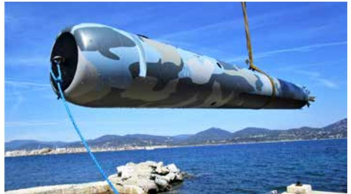
D19 UUV on a F21 torpedo base. (Naval Group photo.)
