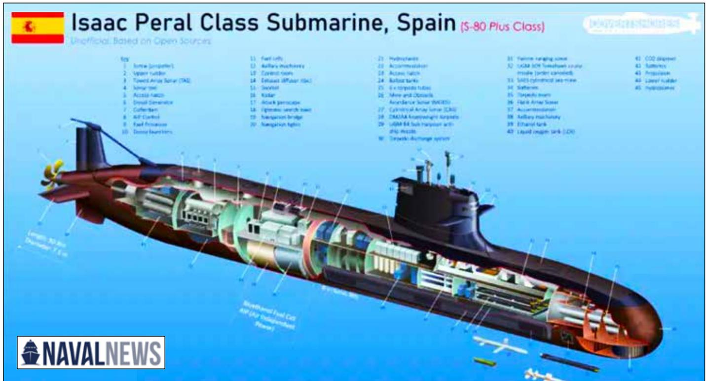
Cutaway of the Spanish Navy's S-80 Plus design is a long-range non-nuclear submarine with Air Independent Power (AIP).
